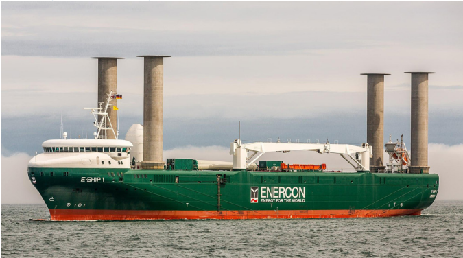
The E-Ship 1 is a Flettner ship: four large rotorsails that rise from its deck are rotated via a mechanical linkage to the ship's propellers. – Alan Jamieson from Aberdeen, Scotland, CC BY 2.0 < https://creativecommons.org/licenses/by/2.0/ >, via Wikimedia Commons
